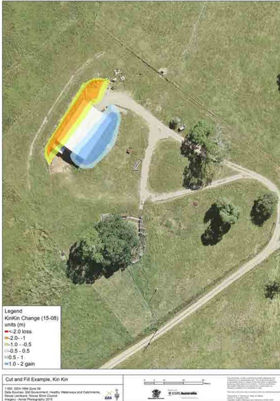
Map 2: Cut and Fill example showing loss of elevation where soil has been removed on slope and then used as fill as gain in elevation to create a level pad for shed/house.
