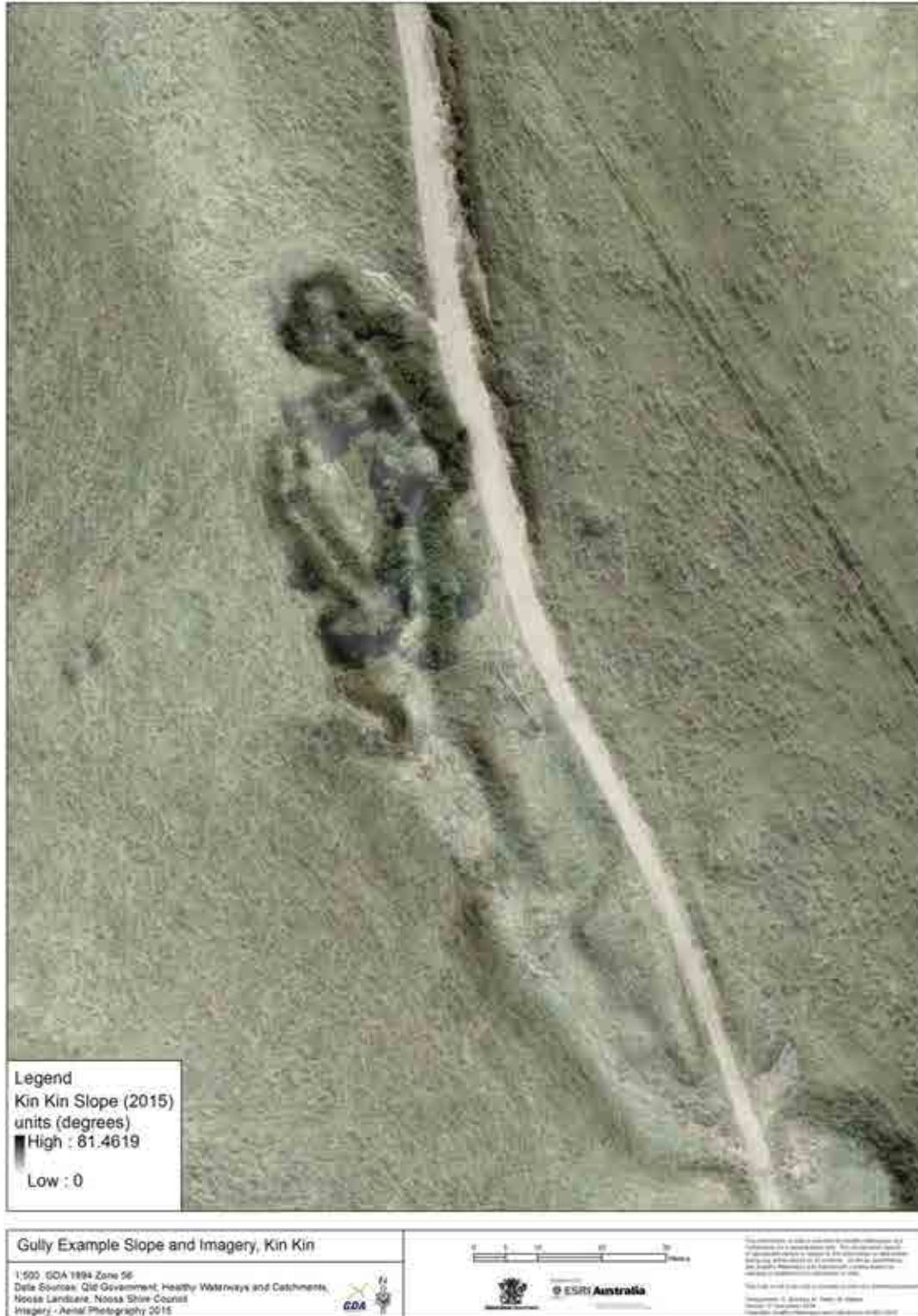
Map 3b: LiDAR slope showing Erosion Type of “gully erosion” where dark slope represents steeper areas and light slope are flatter areas
