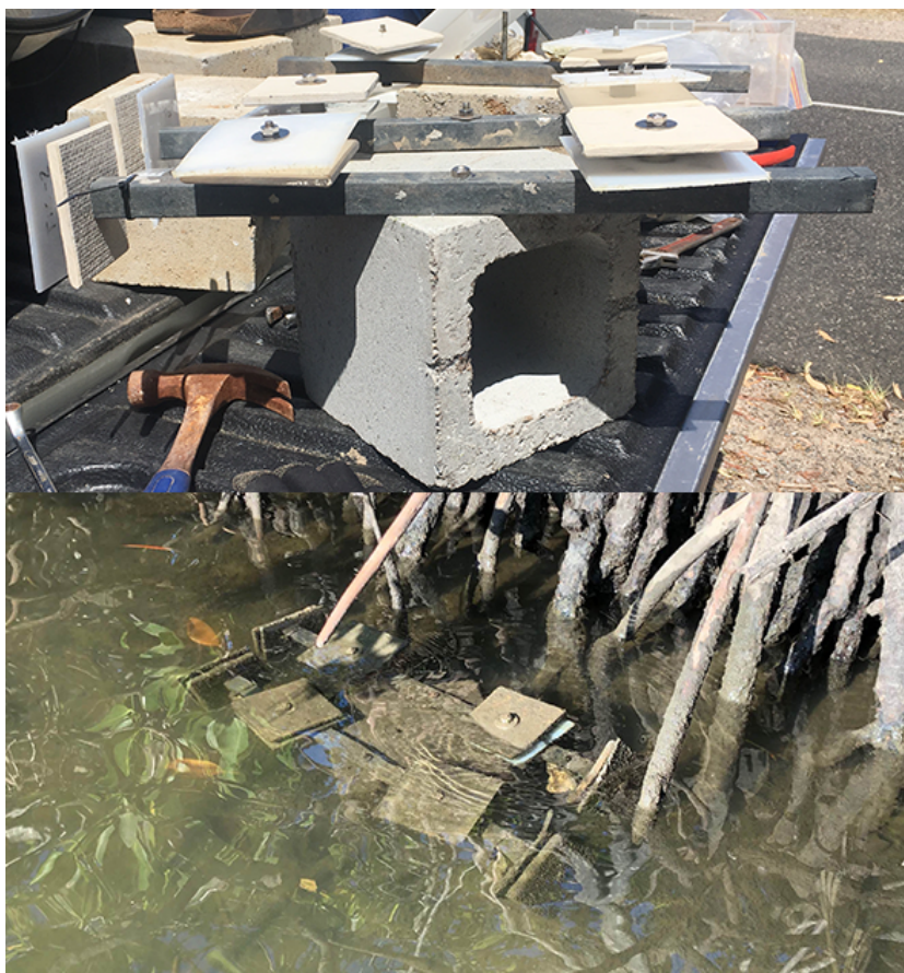
Figure 3. Settlement plate rack design. Top: construction of settlement racks. Bottom: settlement rack in situ at site SD1.
