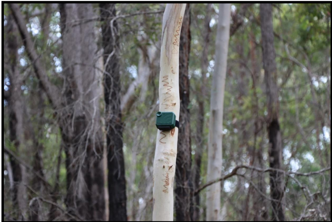
Figure 4: AudioMoth bio acoustic sound recorders installed in Weyba Section Noosa National Park
